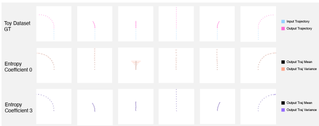
Figure 8: Influence of entropy loss on particle experiment. The input trajectory (cyan, only shown in top row) is identical in all cases. The model trained without an entropy loss term (middle row) covers all modes with high variance, while the model with moderate entropy regularization (bottom row) is able to learn the modes with low variance and without overlap.
