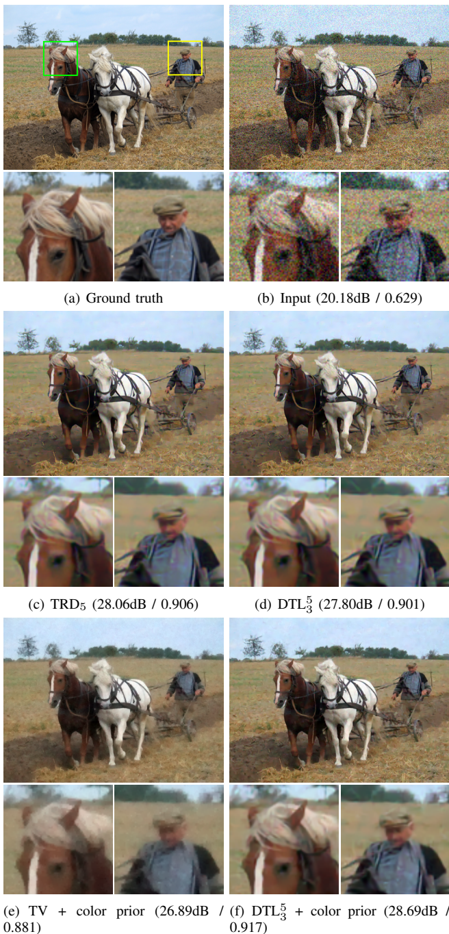
Fig. 10: Experiment on incorporating a color prior [54] with our model after being trained. The input noise level \sigma = 25 . (e,f) show the results of combining total variation (TV) denoising with a cross-channel prior, and our method with a cross-channel prior, respectively. PSNR (dB) and SSIM values are reported inside the bracket of each sub-caption. Please zoom in for better view.
